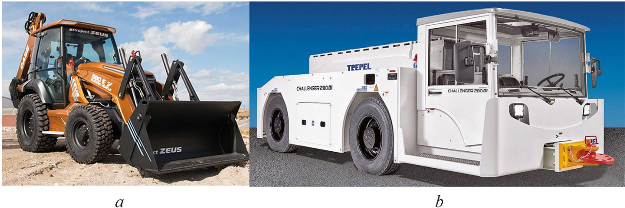
Figure 2 – a ) Electric backhoe loader CASE 580 EV, b ) electric airfield tractor Trepel Challenger 280e for aircraft with a steering mass of 250 tons.
